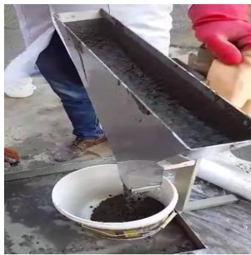
Fig. 2: Rheological parameters of the SCC: (a) Slump flow; (b) V-funnel; (c) L Box test (EFNARC Guidelines., 2005).
