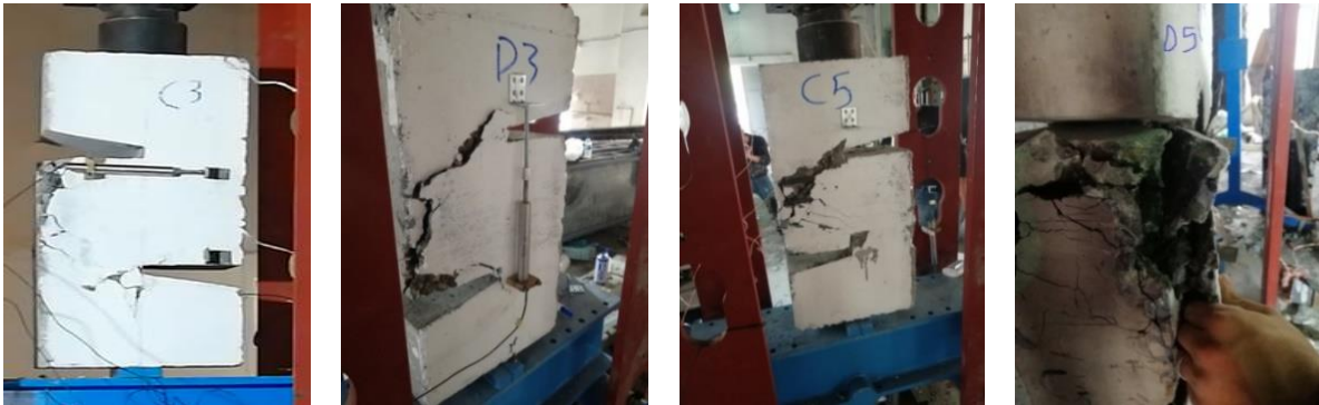
Figure 7 : Specimens C3, D3, C5 and D5 after failure. (Source: Researcher)
