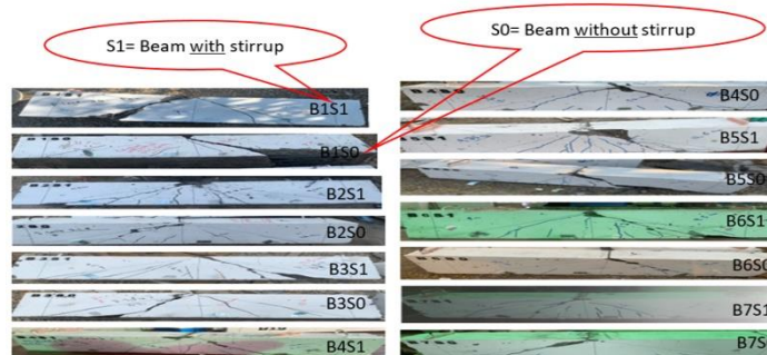
Fig. 5: Crack patterns for beams. (Source: Researcher)
