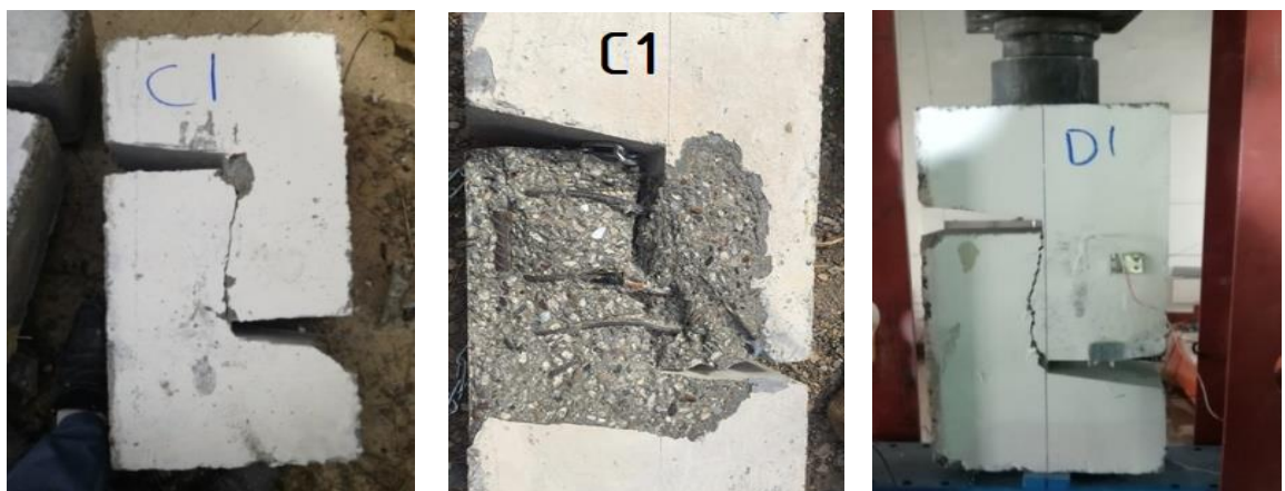
Fig. 5: Specimens C1 and D1 after failure. (Source: Researcher)
