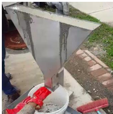
Fig. 2: Rheological parameters of the SCC: (a) Slump flow; (b) V-funnel; (c) L Box test (EFNARC Guidelines., 2005).
